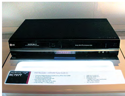
LG's new RC797T combines a digital tuner, DVD and VCR into one unit, equipped with FireWire.
